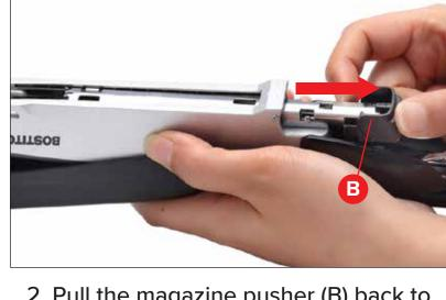
2. Pull the magazine pusher (B) back to expose the staple channel.
