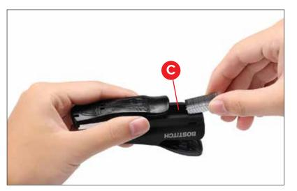
3. With the staple points facing up, drop the staples into the channel (C).
